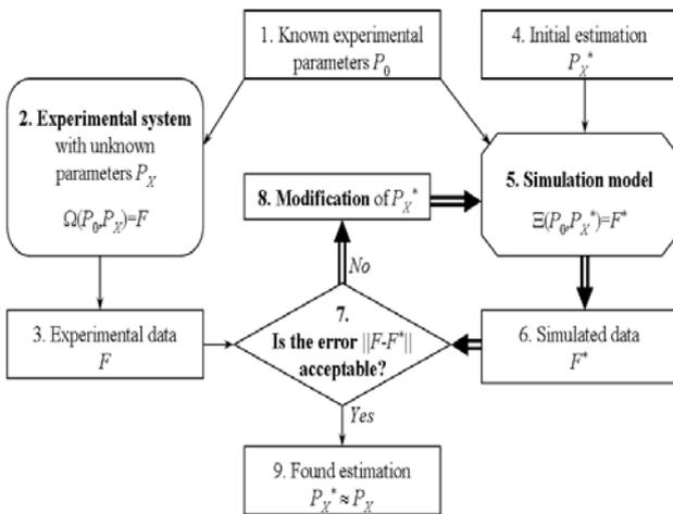
Figure 1. Flow diagram of simulation-based fitting
